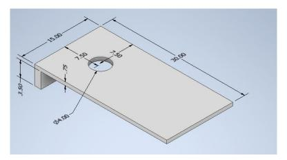
Materials: 3/4" Plywood Wood with 2"x4" attached (1/3 scale cornhole board)
